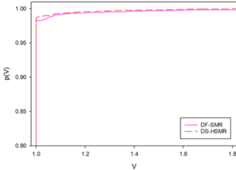
**Figure 3:** Performance profiles based on number of function evaluations (NFE).
