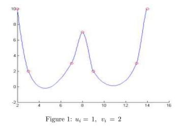
It can be seen that the ordinary spline curve does not guarantee to preserve the shape. Some negative values can be seen in the presentation of the curve. Thus, it is required to assign appropriate values to the shape parameters  $u_i$ ,  $v_i$  so that it generates a curve which preserves the shape of the data. To proceed with this strategy certain mathematical treatment is needed as follows:
