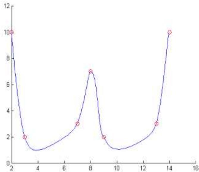
Figure 5: Shape Preserving Rational Cubic Spline curve to the data in Table 1.
