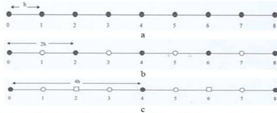
Figure 1: a, b and c Show the Node Points for the Full-, Half-, and Quarter-sweep Cases Respectively
