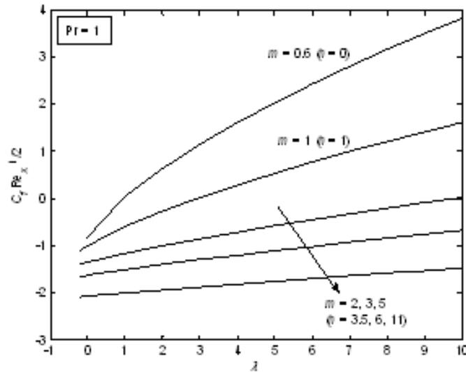
Figure 7: Variation of the Skin Friction Coefficient  $C_f Re_x^{1/2}$  against  $\lambda$  for some values of  $m$  (and  $n$ )
